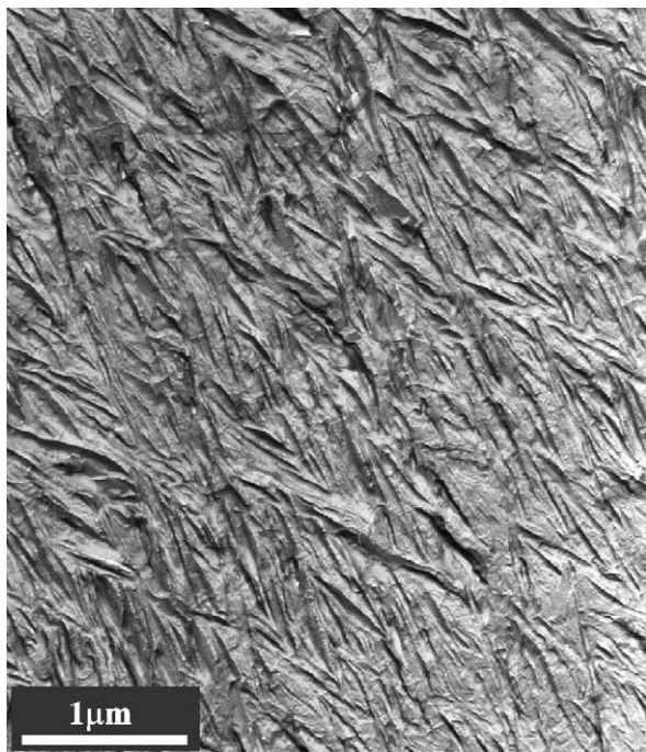
Fig. 2. A replica of the outer edge of a row structure of Sclair 2907 crystallized for 30 min at 128 °C and used for TEM measurements of lamellar thickness with the precautions described in the text.
